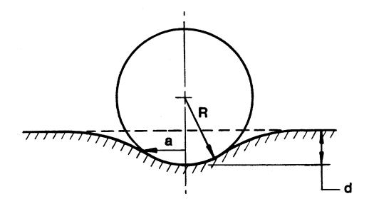
Fig. 2 Cross-sectional view of a hammer-string contact.
