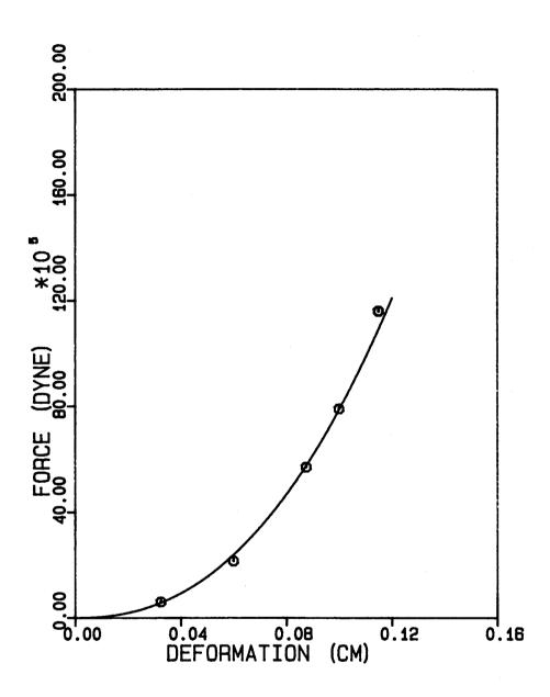
Fig. 4 Force-deformation relationship of a real bass hammer measured by a dynamic method.
