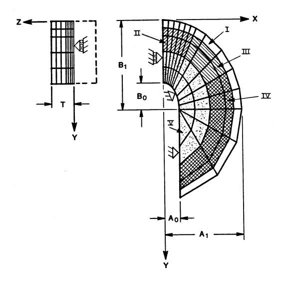
Fig. 1 Finite element model of a piano hammer.
