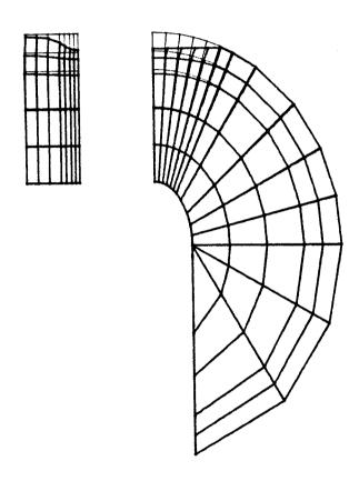
Fig. 5 Deformation of the hammer model for case I and d=0.15cm.
