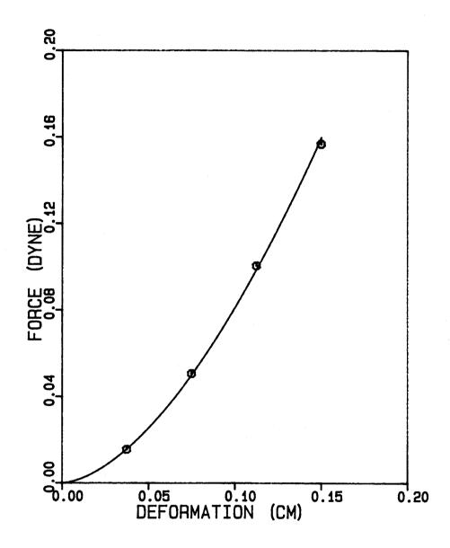
Fig. 3 Force-deformation relationship of the hammer model for case I.
